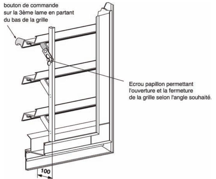
OUVERTURE/FERMETURE PAR VÉRIN MANUEL EN FACE ARRIÈRE
