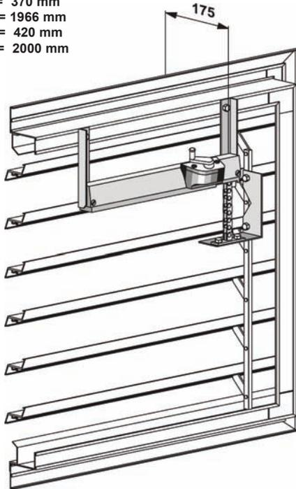
OUVERTURE/FERMETURE RÉGLABLE MANUELLEMENT
