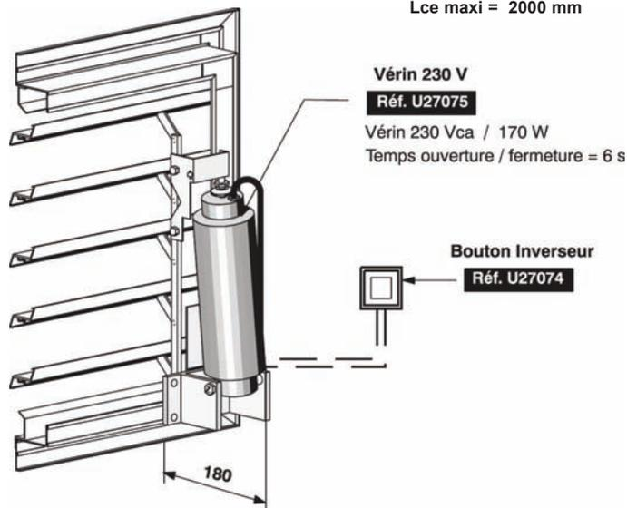
OUVERTURE / FERMETURE "TOUT OU RIEN" PAR SERVOMOTEUR AVEC RESSORT DE RAPPEL
